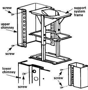
Position upper chimney section on support system frame.
